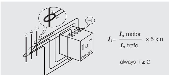
$$I_B = \frac{I_N \text{ motor}}{I_N \text{ trafo}} \times 5 \times n$$
